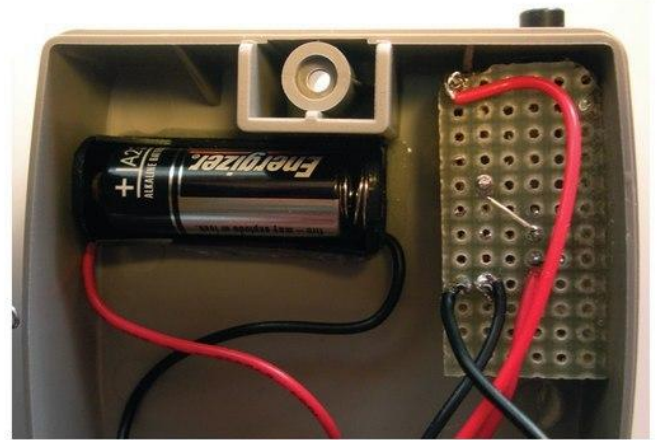
■ FIGURE 7. Installed battery and PCB.
